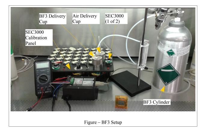
Only one of two SEC3000 units used in the tests can be seen in the Figure. The other is covered by the air delivery cup. Also in the Figure, the BF3 delivery cup has been moved to the front of the calibration panel, maintaining approximately the desired bend in the PTFE tubing, which is not very flexible.
