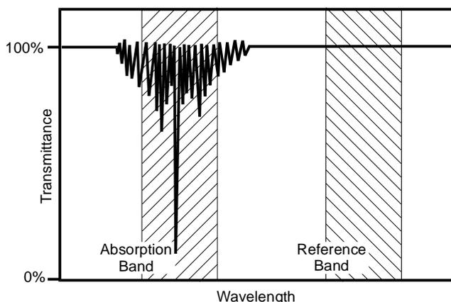
The dual channel receiver is a single wafer, double filtered, dual receiver with an internal optical barrier. The elements are perfectly matched resulting in overall stability and superior performance throughout the entire temperature range.
