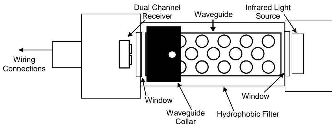
Using a dual channel receiver there is no need to use any special lenses or beam splitters to achieve the different measurement bands.
