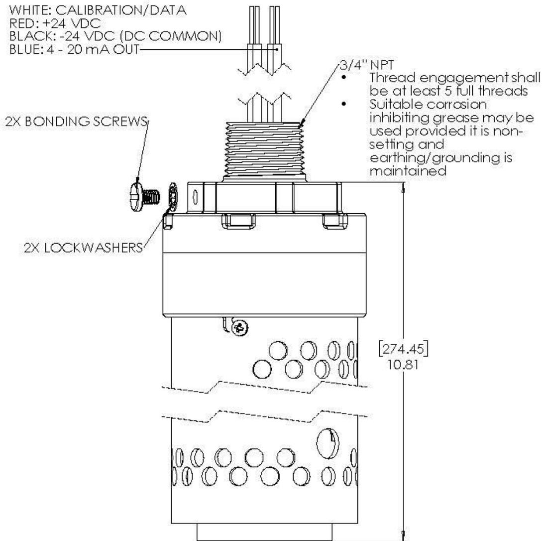
1. LOCKWASHERS REQUIRED IF BONDING SCREWS USED FOR GROUNDING TO ENSURE THE WIRE WILL NOT COME LOOSE
