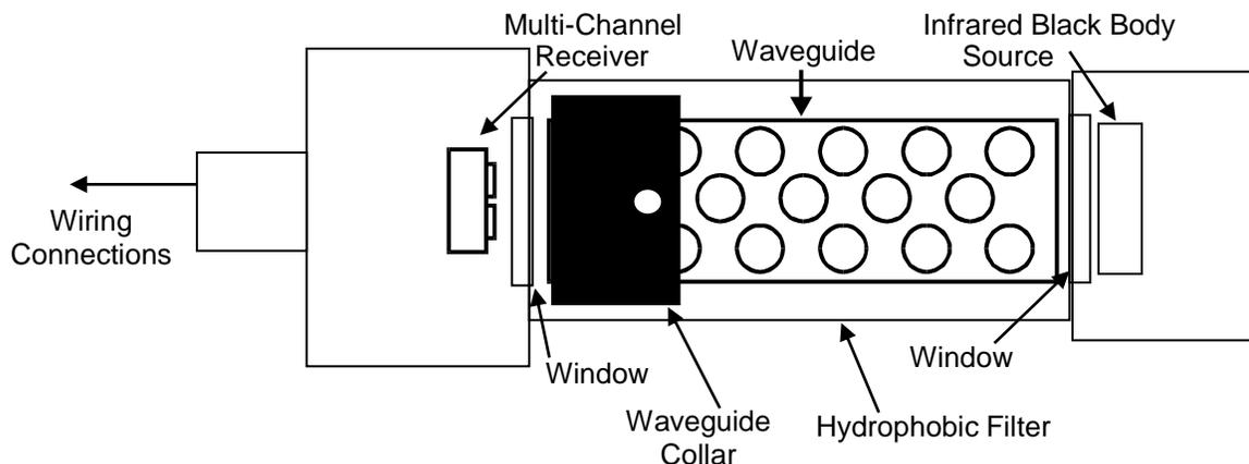
The straight line optical system eliminates the need for any special lenses or beam splitters.
