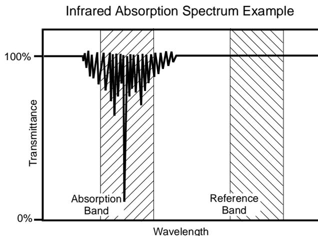
The multiple-channel receiver consists of several filtered light sensors monitoring light bands critical to the target gas. The multi-channel design affords high sensitivity, high selectivity, excellent drift control and superior thermal stability over the entire temperature range.
