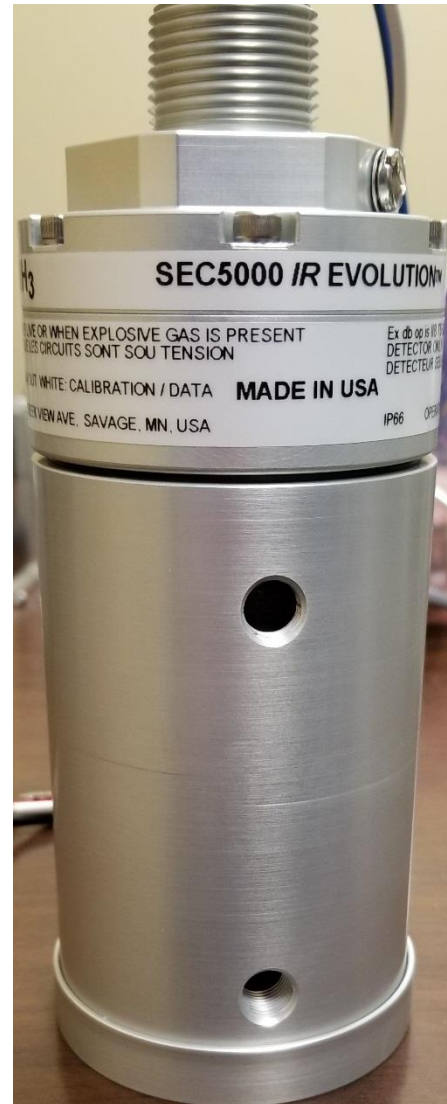
Figure 2 – Final Assembly with the Sample Draw Barrel
