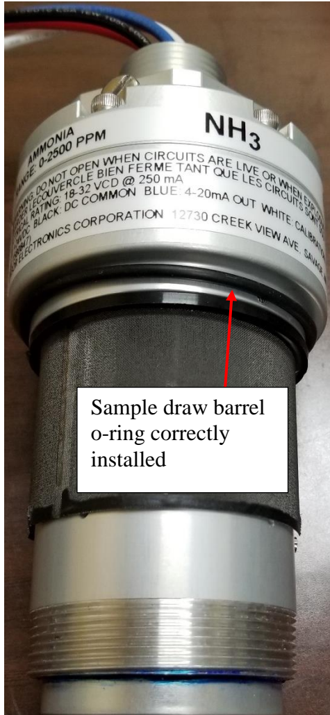
Figure 3 – Sample Draw Barrel O-Ring in Place
