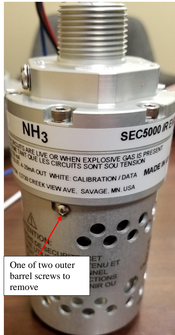
Figure 1 – Unit as Shipped with Original Outer Barrel
