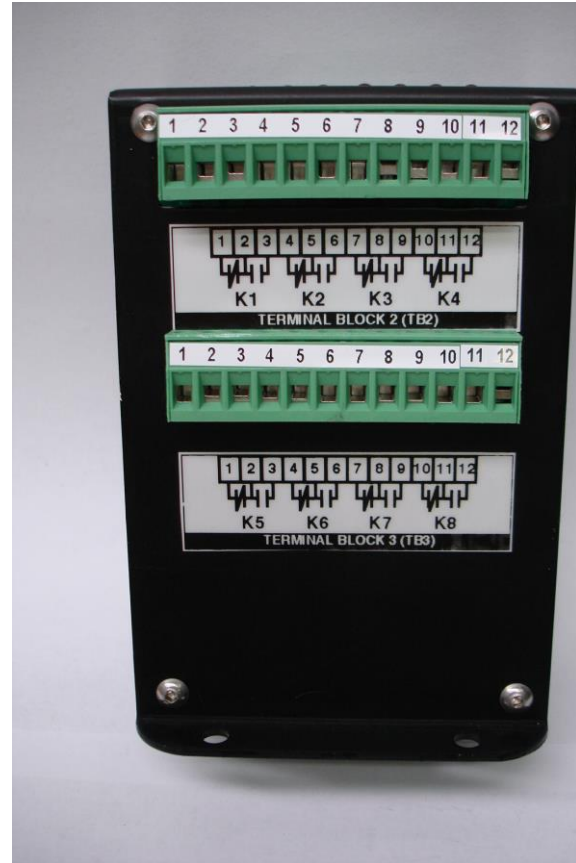
TB 2 AND TB 3 (RELAY CONTACT WIRING)
