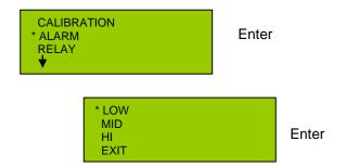
Select the Alarm Relay (LOW, MID, HI) using the down arrow. Once the cursor is on the alarm relay you wish to configure, hold the magnet over Enter. The example LOW will be used. The same operations can be used to set the MID or HI relays.
