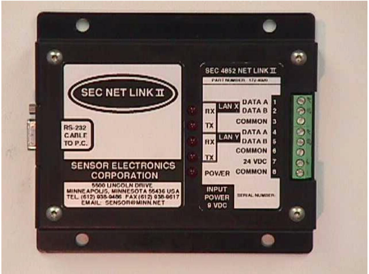
The Net Link II connects to a 9-Pin Din serial port on the PC and has two (2) RS-485 ports available for the SEC network units. The Net Link II can be connected to the data highway in various system configurations. Refer to the Net Link II data sheet for data highway connection and operation. The Net Link II can be powered from the same power source (24VDC) as the SEC field devices **or** with the 9-volt transformer.
