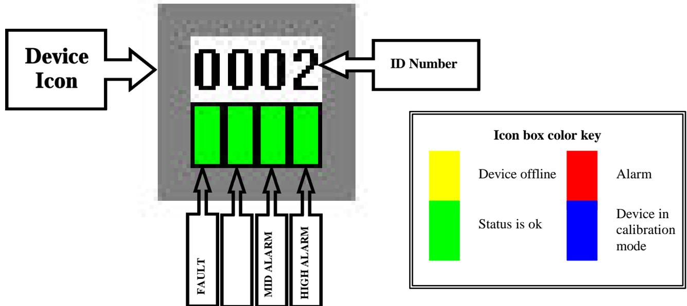
Each icon has a unique identification number. The icon has four boxes that will change colors for various conditions allowing the operator to see at a glance if any device is in alarm or fault. Each device has a data file that is continuously updated and stores the information on the computer's hard drive. The stored information can be viewed, graphed and printed for hard copy reports.
